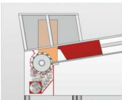
Rotor with diameter 354 mm for higher throughput
