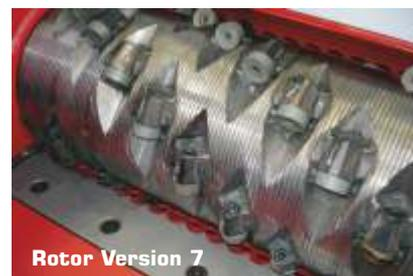
The use of various types of knives enables job-related adjustment of the shredder to the material being processed.
