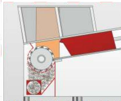
Rotor with diameter 482 mm with very high throughput
